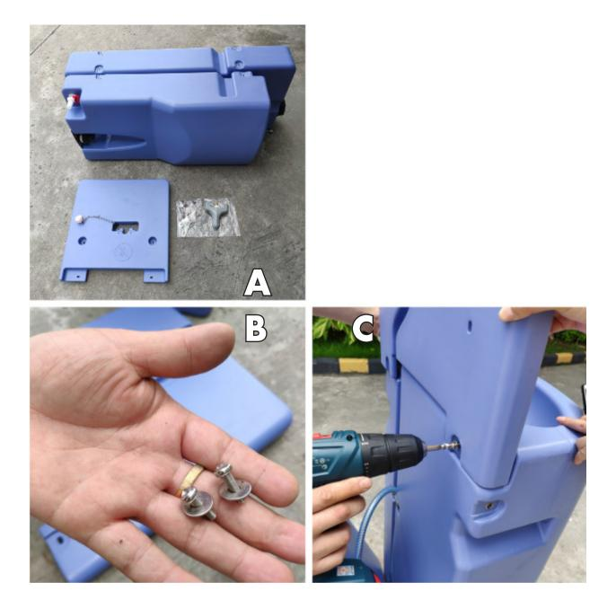
1. Attach back panel to the waste tank. This will require two screws. Be sure to insert the back panel with the screw holes facing the back of the unit, as shown.
