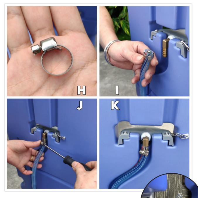
3. Connect inlet water pipe to water tap on back of the unit. To do this, slide adjustable clamp over the top of the pipe, then align mouth to the tap. Then, tighten clamp to secure the connection. Inlet water pipe is located at the bottom of the waste water tank, attached to the foot pump.
