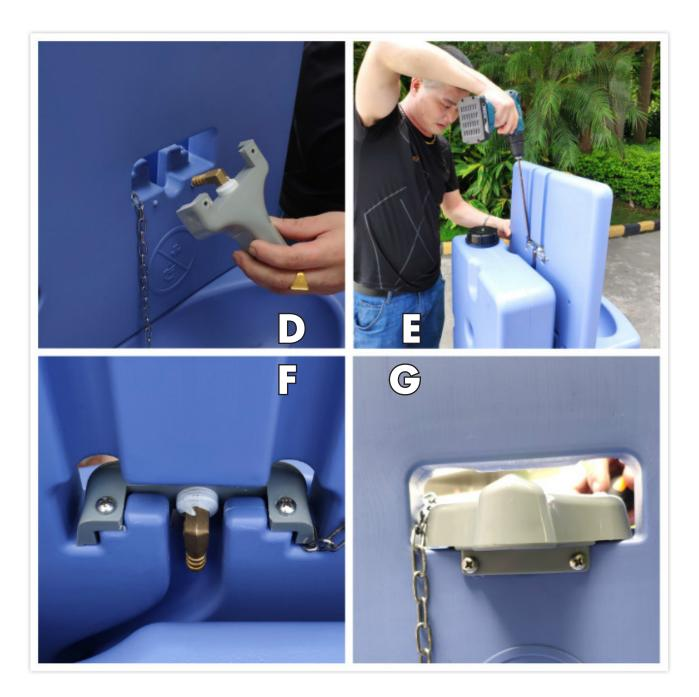
2. Using a drill, affix the tap on the back panel. This will require four screws. (Figs. G and H demonstrate the front and back of the tap.)
